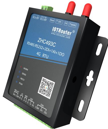
ZHC493C is a support2Road dry (wet) node detection,1Relay (COM, NO) output,1Analog quantity (current 4~20mA) detection, 1 channelRS485 pass through, 1 way RS232 transparent transmission. The latest network IO products are compatible with Modbus RTU/TCP protocol. With "remote control" as the core function, it is highly easy to use, and users can easily and quickly integrate into their own systems to realize LTE, RS485Remote and loca lcontrol.
